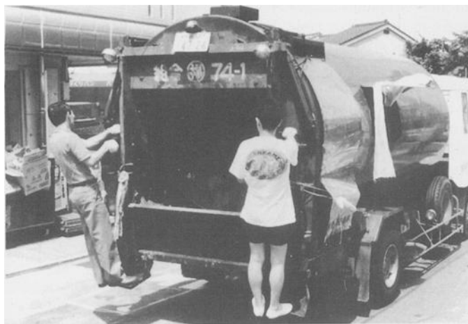
FIG. 1—Garbage truck of the same type involved in the accident, showing two men on the foothold and between them, the entrance to the drum.
